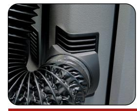
CaliHeat mounting at the bottom of the air vent for VW Camper with outlet grille in the B-pillar.
